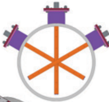
VAP 3 Pitots Circular Duct Installation (front view)
